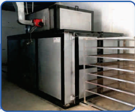
DIESEL FIRED OVEN
